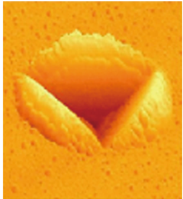
The formed indentation when a pyramid-shaped diamond indenter is pressed into material surface in measuring the hardness of a material.
